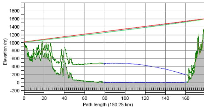
Figure 2. Microwave Path Profile showing antenna centerlines and path clearance over effective Earth's curvature.
