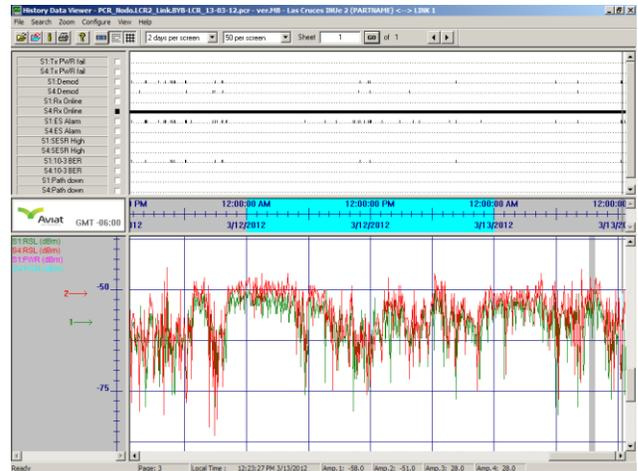
Figure 5. PCR output over 72 hours showing RSL fluctuations but zero Rx alarms.
