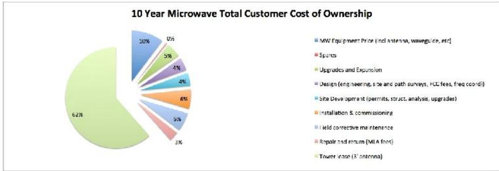
**Figure 1. Tower costs make up the lion's share of the total cost of ownership of microwave backhaul. Reducing antennas sizes would reduce the tower cost for about a 20 percent reduction in total cost.**
