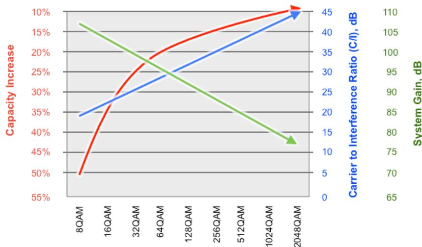
Figure 1: Effect on System Gain and C/I with increasing Modulation
